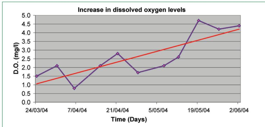
Figure 3. Redline increasing levels of DO.
