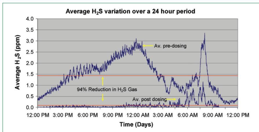
Figure 2. Redlines are the average readings before and after showing a 94% reduction in H<sub>2</sub>S gas.
